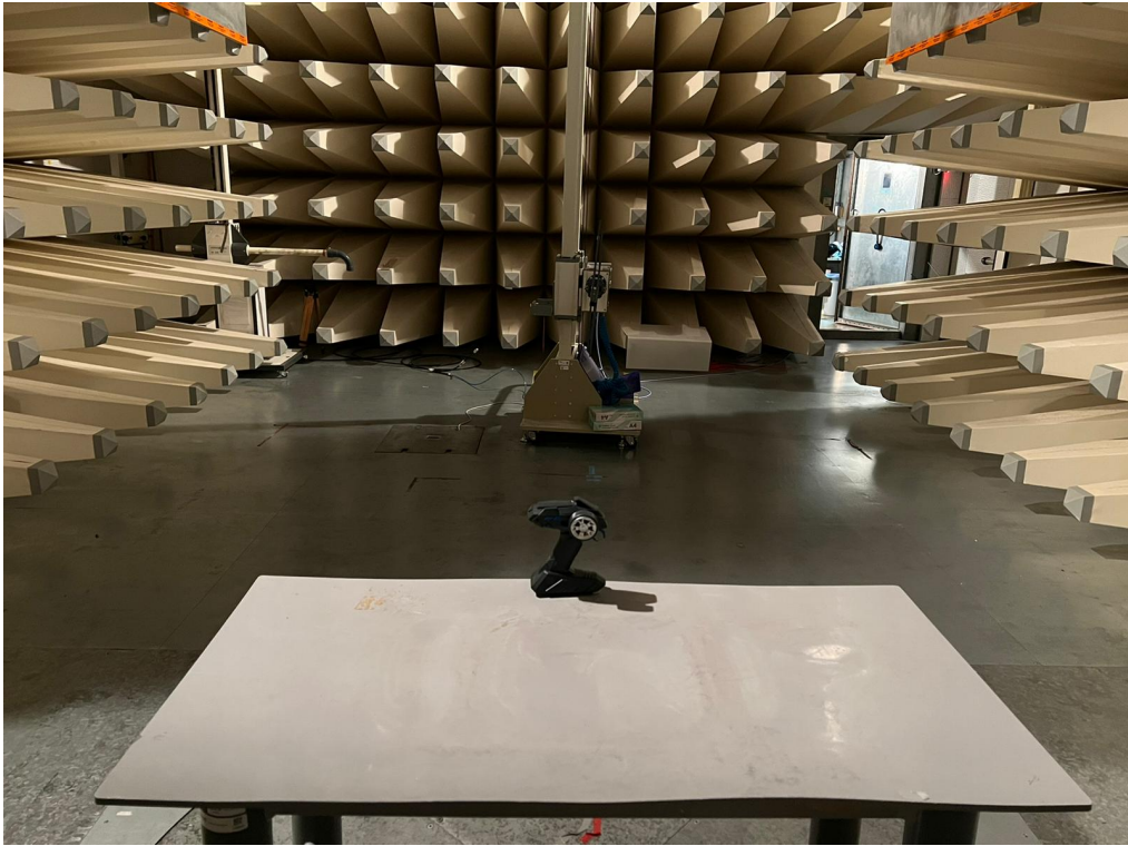
Set-up for Radiated Emission (200-1000MHz)
