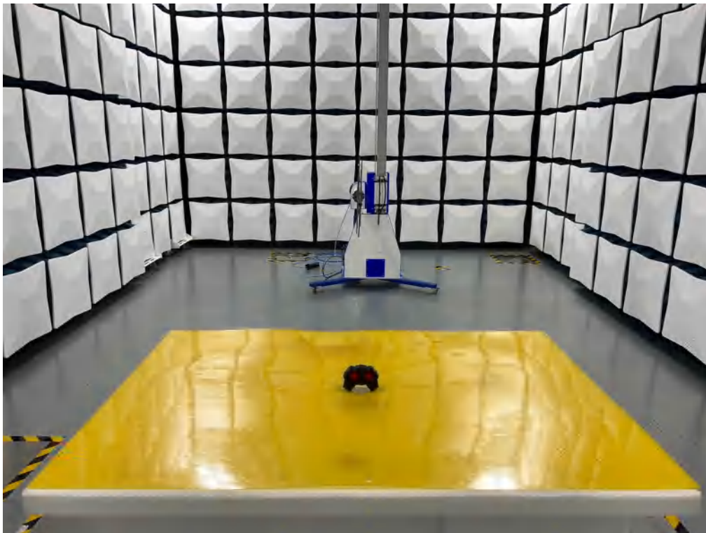
Set-up for Radiated Emission (200-1000MHz)
