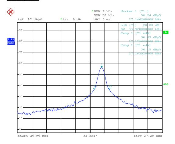
The field strength of any emission within the operation band did not exceed 80 dB ( $\mu$ V/m) for average value or 100 dB ( $\mu$ V/m) for peak value.
