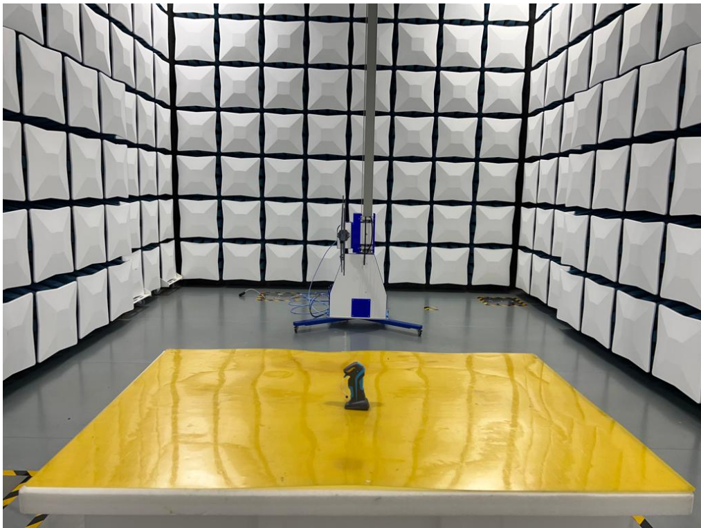
Set-up for Radiated Emission (200-1000MHz)
