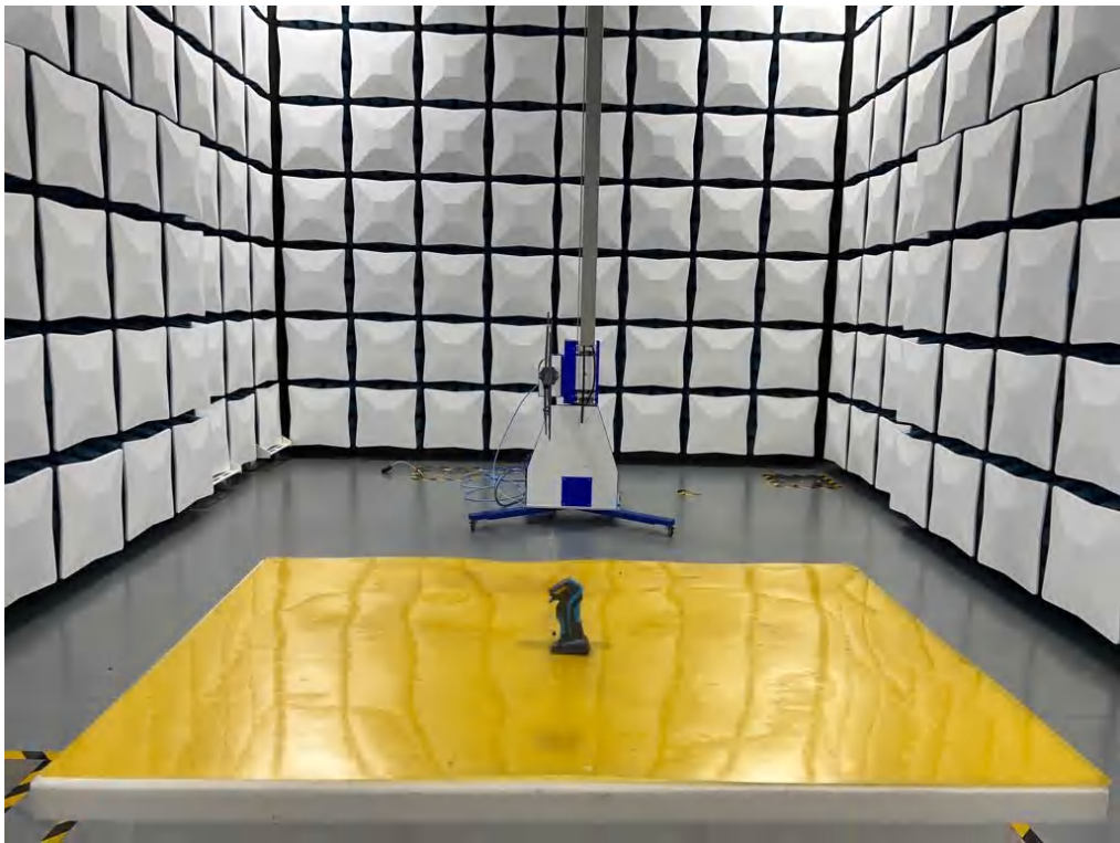
Set-up for Radiated Emission (200-1000MHz)
