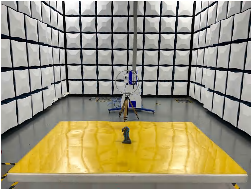
Set-up for Radiated Emission (9k-30MHz)
