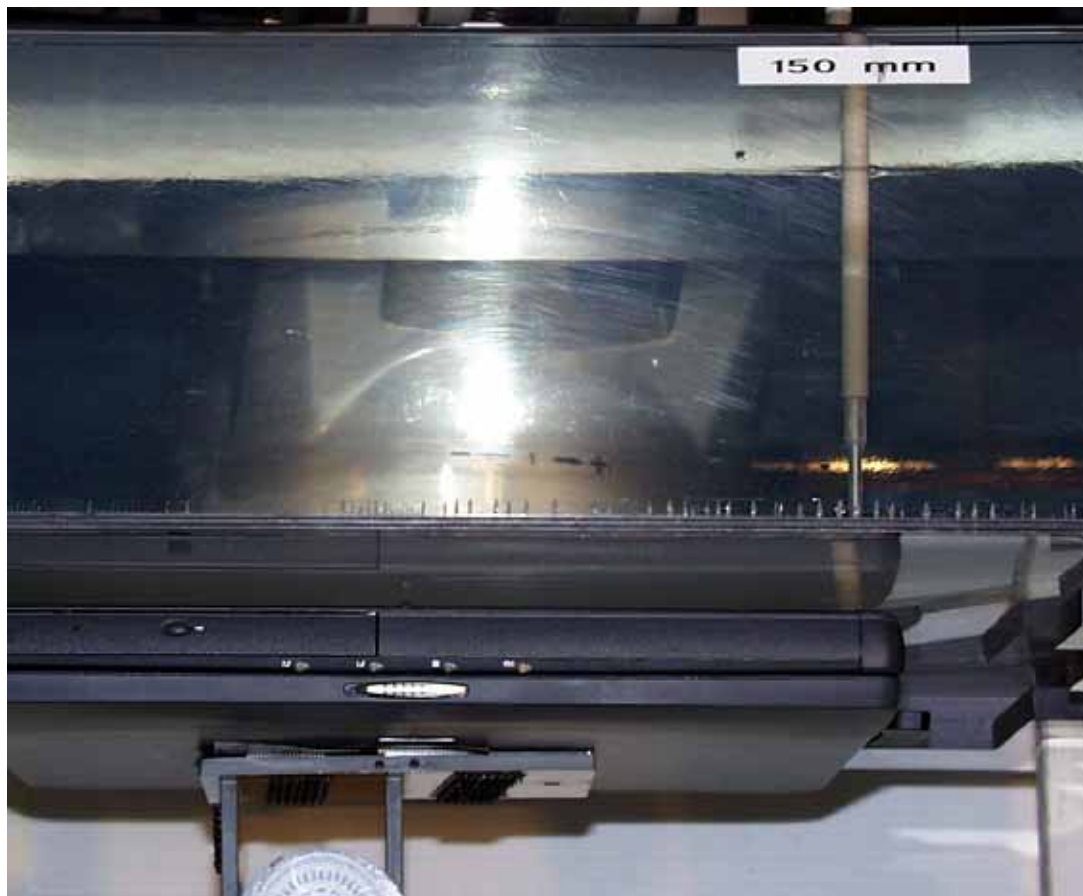
< Bottom of the host PC faced toward the phantom (lap-top position) – 8 mm(Card-to-Bottom) >
