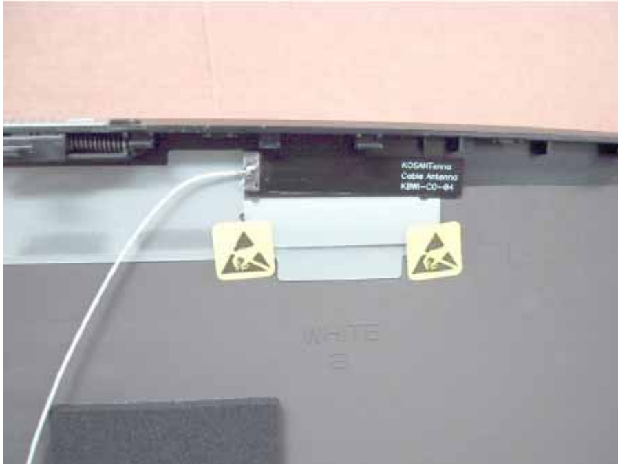
< 2.4 GHz / 5 GHz Dual band KOSAN WLAN antenna (M/N: KBWI-CO-04) >
