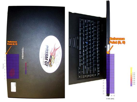
For laptop position (bottom of the host PC against the phantom), we did simple manual prescan in the air at this configuration and there was no field found to be measurable at all since there was at least 15 mm separation distance between the antenna and the bottom of the host PC. Refer to the location of the antenna mounted inside the host PC below.
