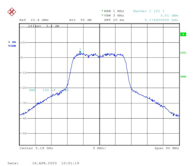
Plot 33 - Peak power spectral density (conducted) in any 1 MHz band.
