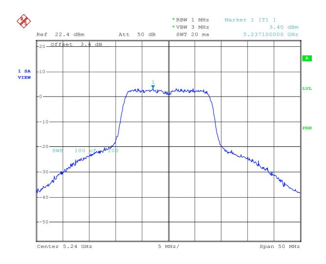
Plot 22 - Peak power spectral density (conducted) in any 1 MHz band.
