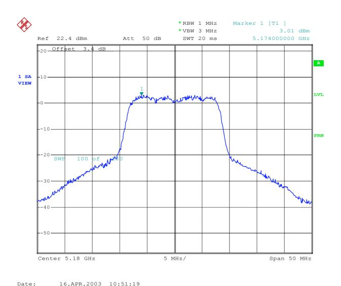
Plot 17 - Peak power spectral density (conducted) in any 1 MHz band.
