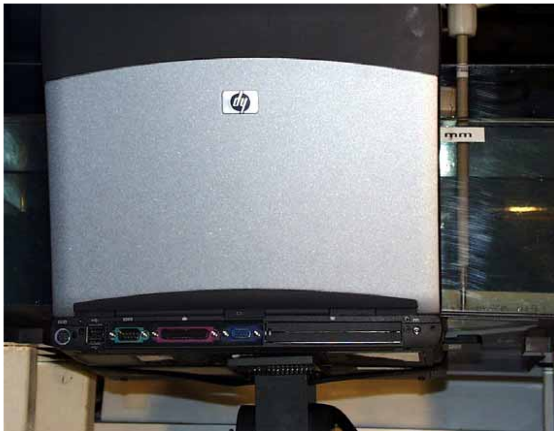
< Top (Keyboard) of the host PC faced toward the phantom – 5 mm(Card-to-Top) >
