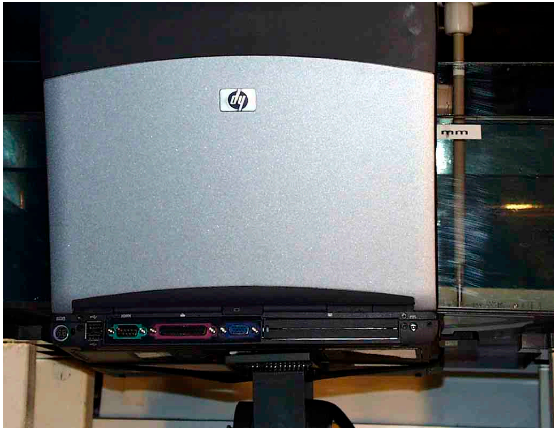
< Top (Keyboard) of the host PC faced toward the phantom – 5 mm(Card-to-Top) + \alpha mm >
