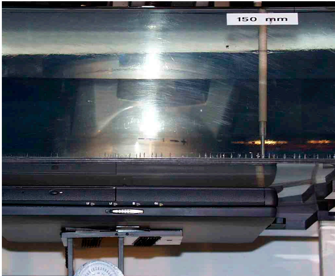
< Bottom of the host PC faced toward the phantom (lap-top position) – 8 mm (Card-to-Bottom) + \alpha mm >
