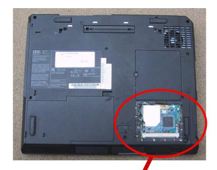
Detail of ISL38001M card mounted miniPCI slot of IBM R30
