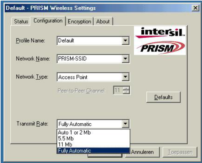
fig. 04: WLAN tx rate setting window
