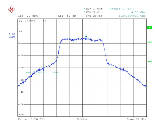
Plot 44 - Peak power spectral density (conducted) in any 1 MHz band.
