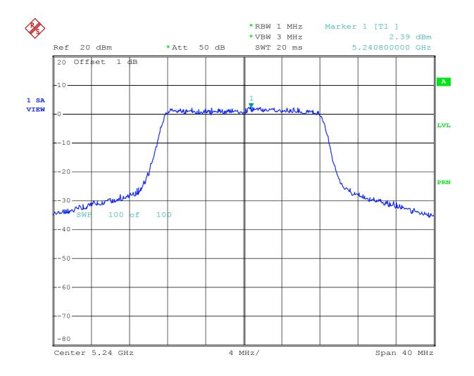
Plot 38 - Peak power spectral density (conducted) in any 1 MHz band.
