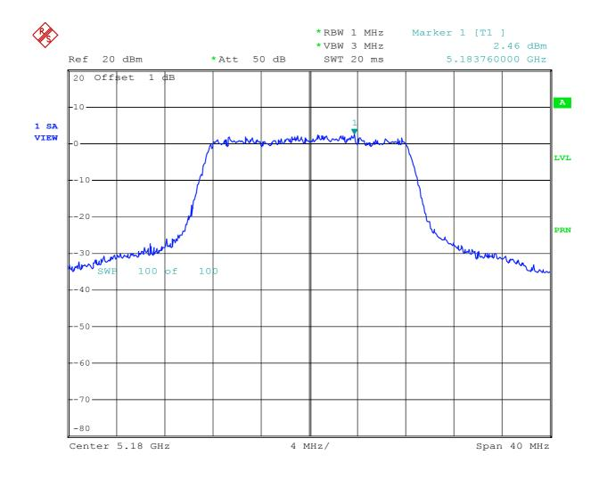
Plot 36 - Peak power spectral density (conducted) in any 1 MHz band.
