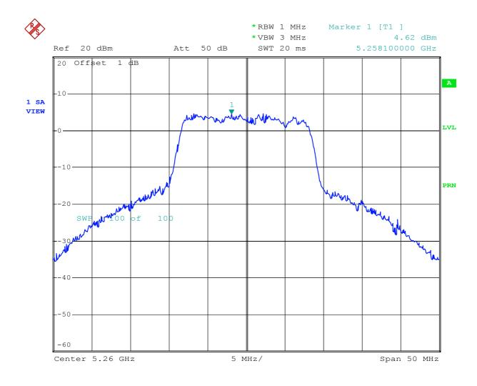
Plot 41 - Peak power spectral density (conducted) in any 1 MHz band.
