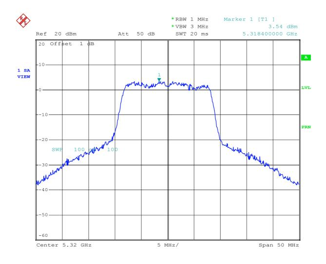
Plot 48 - Peak power spectral density (conducted) in any 1 MHz band.
