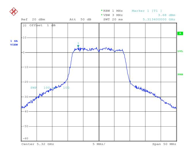
Plot 47 - Peak power spectral density (conducted) in any 1 MHz band.
