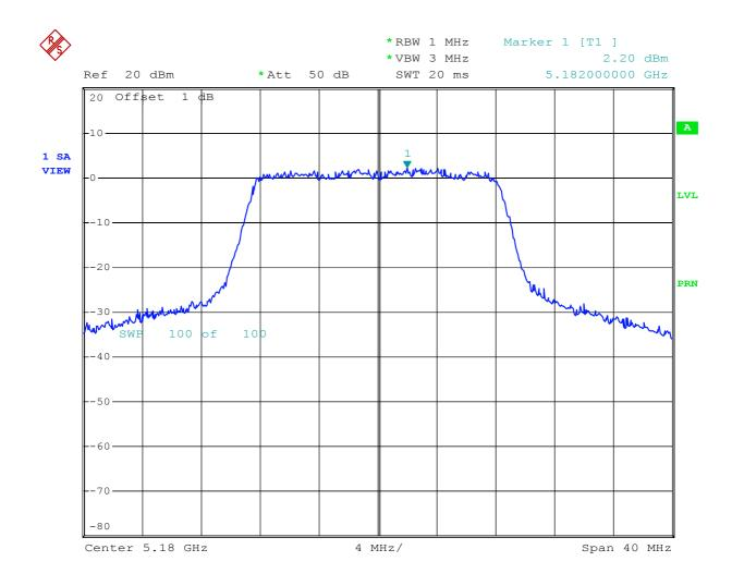
Plot 35 - Peak power spectral density (conducted) in any 1 MHz band.
