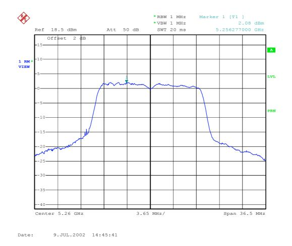
Plot 9 - Peak power spectral density (conducted) in any 1 MHz band.
