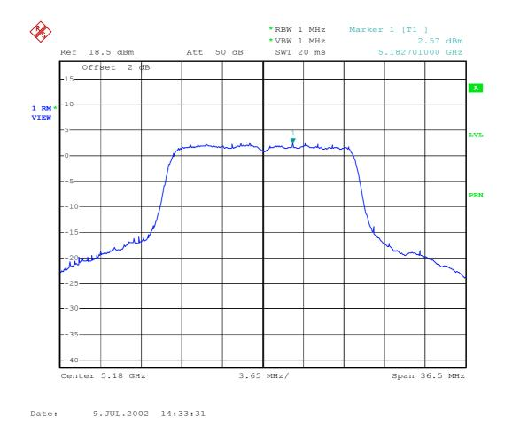
Plot 4 - Peak power spectral density (conducted) in any 1 MHz band.
