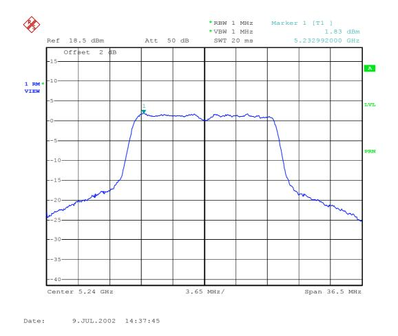
Plot 6 - Peak power spectral density (conducted) in any 1 MHz band.
