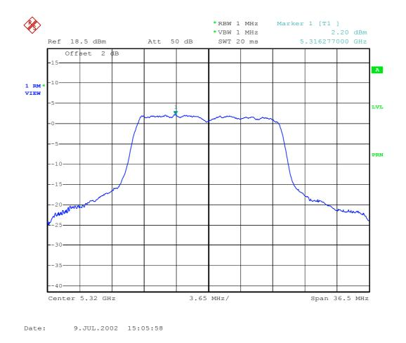
Plot 15 - Peak power spectral density (conducted) in any 1 MHz band.
