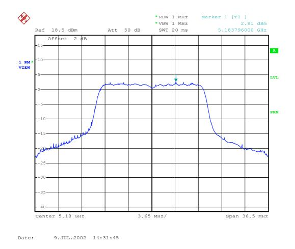
Plot 3 - Peak power spectral density (conducted) in any 1 MHz band.
