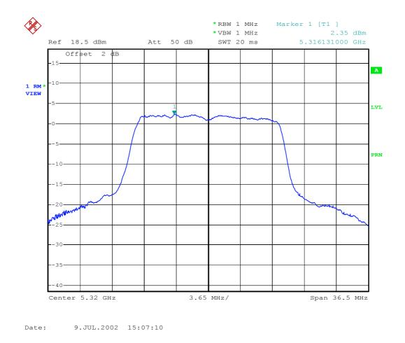
Plot 16 - Peak power spectral density (conducted) in any 1 MHz band.
