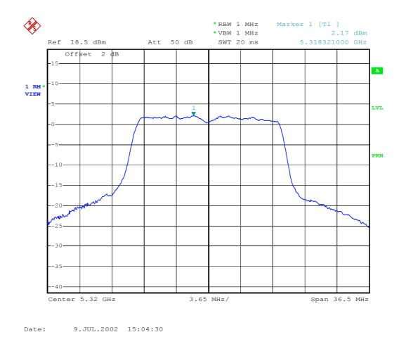
Plot 14 - Peak power spectral density (conducted) in any 1 MHz band.
