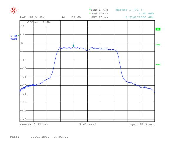
Plot 13 - Peak power spectral density (conducted) in any 1 MHz band.
