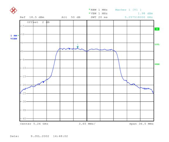
Plot 11 - Peak power spectral density (conducted) in any 1 MHz band.
