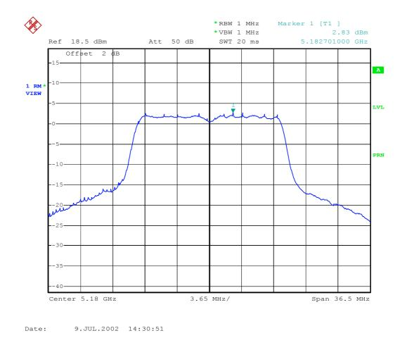
Plot 2 - Peak power spectral density (conducted) in any 1 MHz band.
