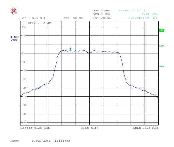
Plot 10 - Peak power spectral density (conducted) in any 1 MHz band.
