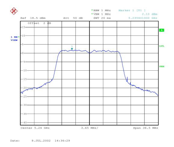
Plot 5 - Peak power spectral density (conducted) in any 1 MHz band.
