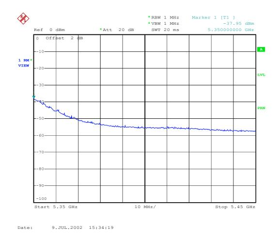
Plot 30 – Emissions in the 5.35 – 5.46 GHz restricted band of operation
