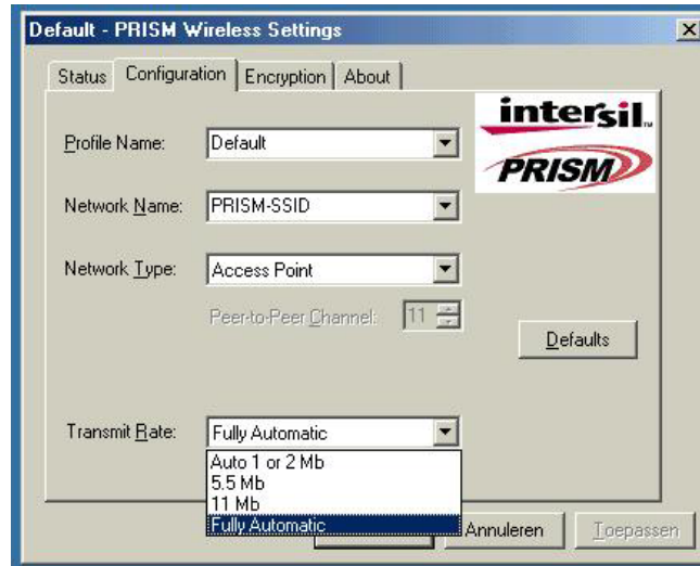
fig. 04: WLAN tx rate setting window
