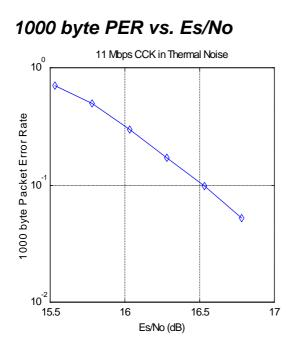
The reference PER is specified as 8%. The corresponding Es/No (signal to noise ratio per symbol) is 16.4 dB. The Es/No required to achieve the desired BER with maximum system implementation losses is 18.4 dB. The minimum processing gain is again, 10 dB, therefore:
