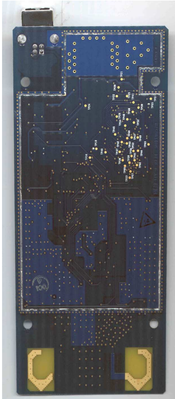
ISL37300XU PCB Rear view without shields (RF)
