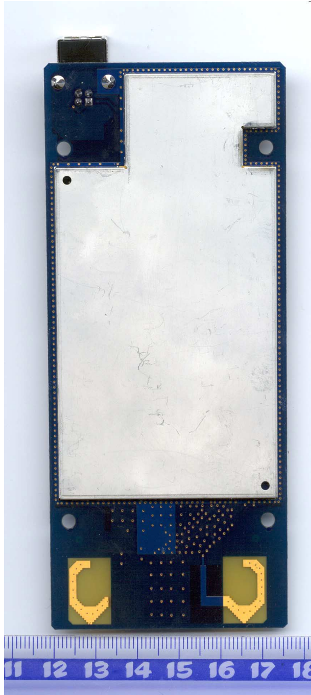
ISL37300XU PCB Rear view with shields (RF)
