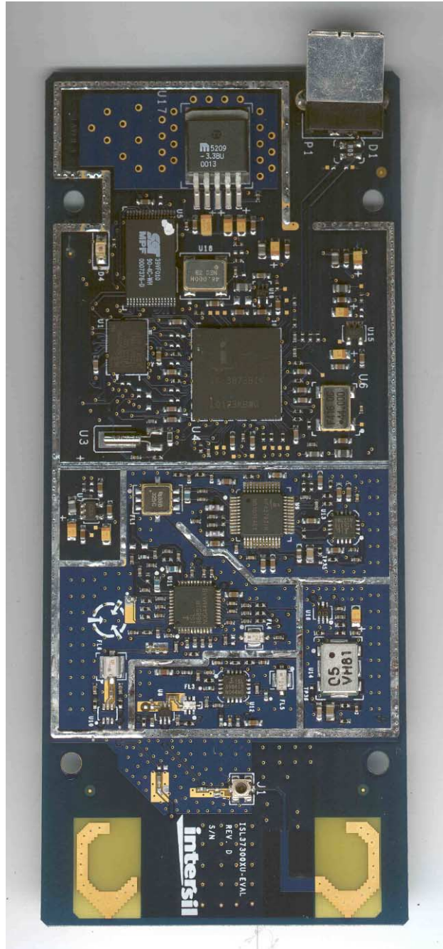
ISL37300XU PCB front view without shields
