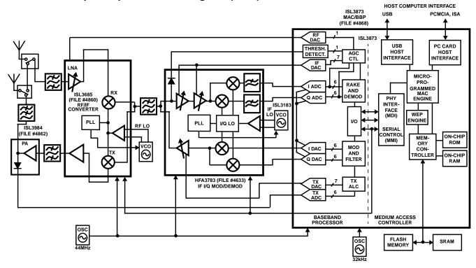
PRISM 2.5 11Mbps Chip Set Block Diagram (PCI)
