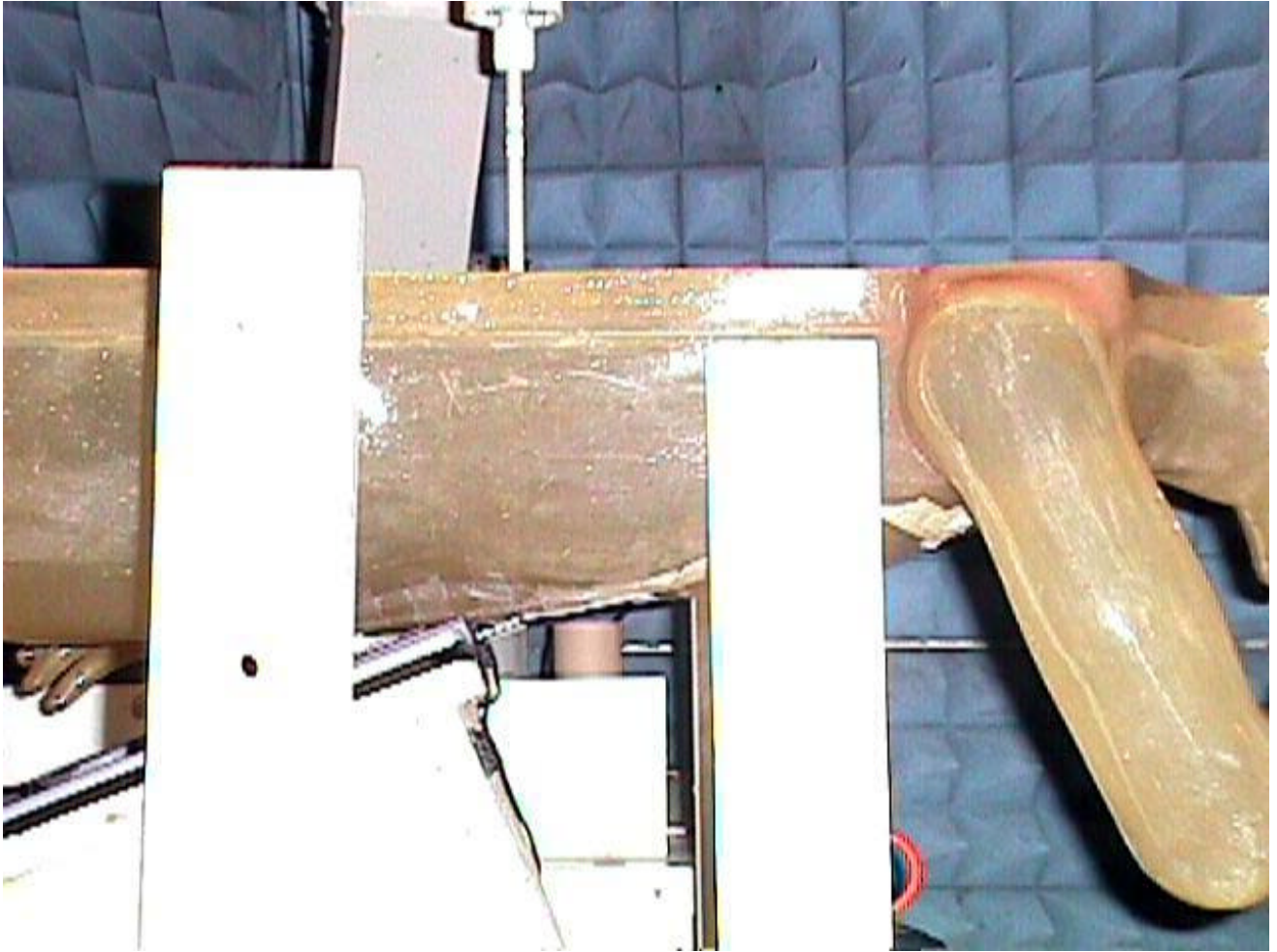
< Overview – Tip of the EUT in contact with the phantom and the display of the laptop outward from the phantom >
