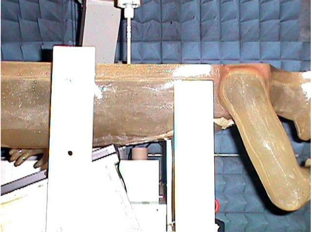
< Overview – Tip of the EUT in contact with the phantom and the display of the laptop inward to the phantom >
