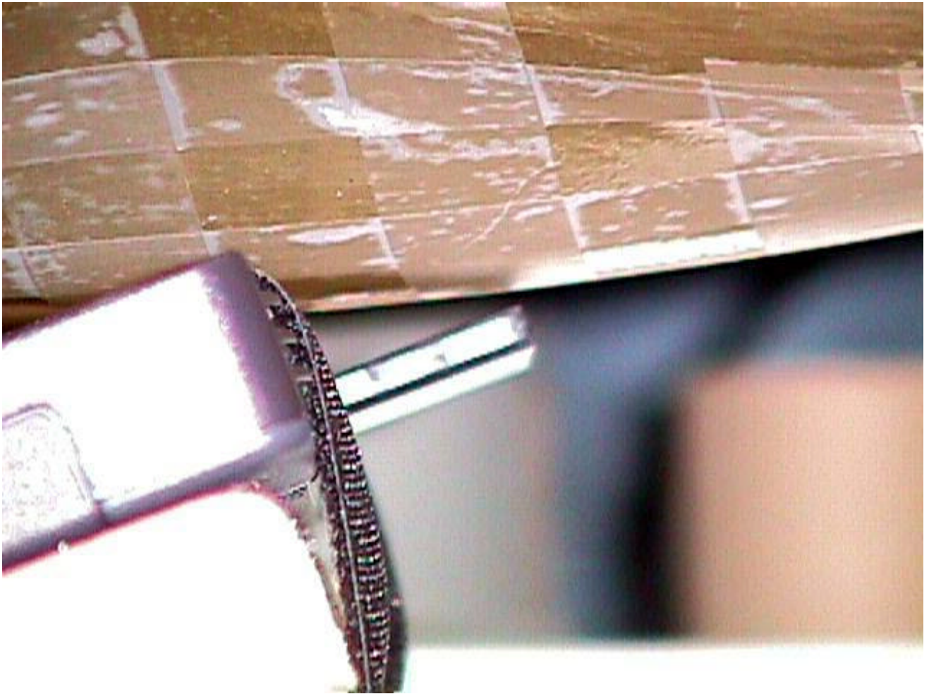
< Close-up view – Tip of the EUT in contact with the phantom and the display of the laptop inward to the phantom >
