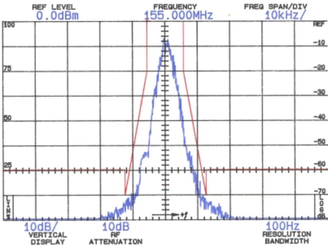
(1) On any frequency from the center of the authorized bandwidth  $f_o$  to 5.625 kHz removed from  $f_o$ : Zero dB 0
