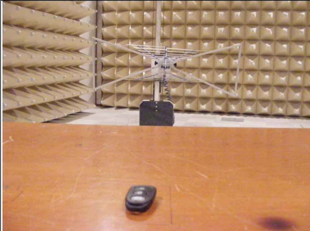
Photo of Field Strength & Spurious Emission Test
