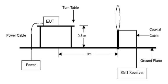
The diagram below shows the test setup that is utilized to make the measurements for emission from 30 \( \mathref{Mt} \) to 1 \( \mathref{Mt} \) Emissions.
