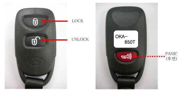
You can lock and unlock your vehicle with the remote transmitter.
