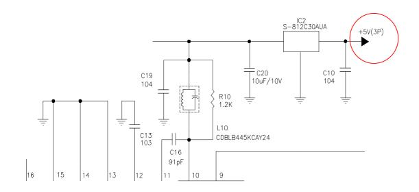
1 portion is a portion which always supplies 5V through DC/DC conversion from Car Battery.
