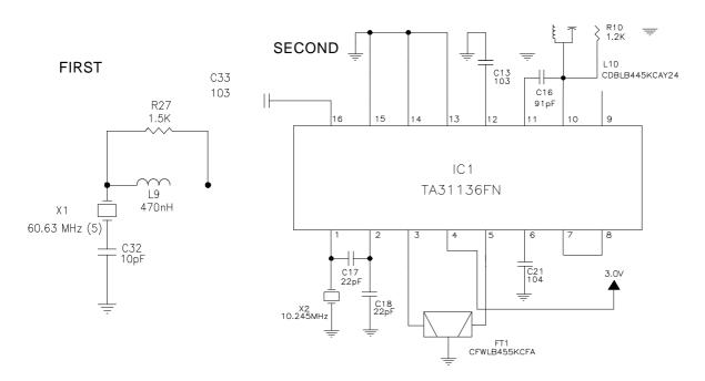
FM oscilation section oscillates with , first oscilation is 60.63 MHz X-Tal Frequency, second oscilation is 10.245 MHz X-Tal Frequency, by the FSK modulation method, FM bands of frequency which is required for FM frequency transmission.
