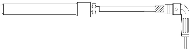
Antenna is composed with Wire Coil Antenna-Jack , and radiates radio frequency through the air.
