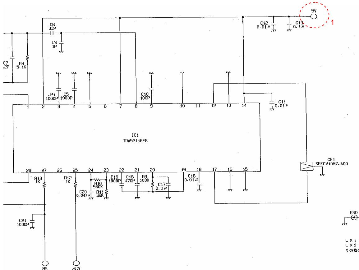
1 portion is a portion which always supplies 5V through DC/DC conversion from Car Battery.
