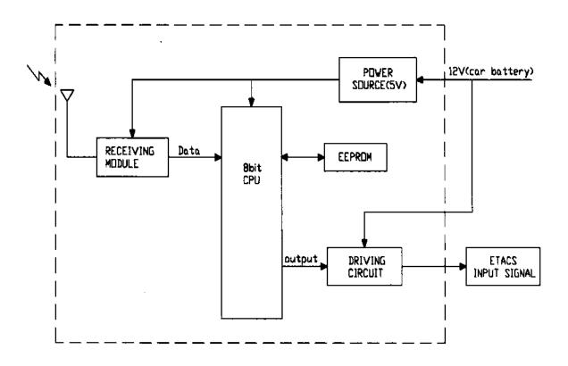
figure 3.1 block diagram of the receiver
