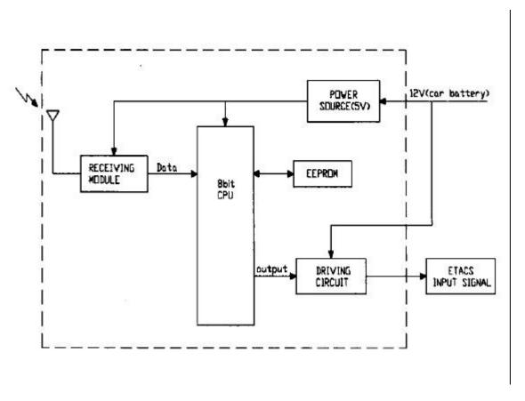
figure 3.1 block diagram of the receiver
