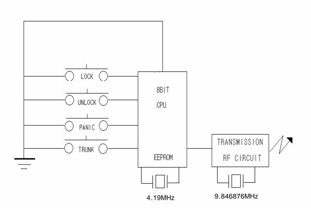
figure 3.1 block diagram of the transmitter
