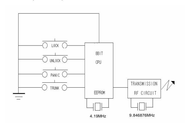
figure 3.1 block diagram of the transmitter
