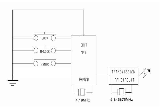
figure 3.1 block diagram of the transmitter
