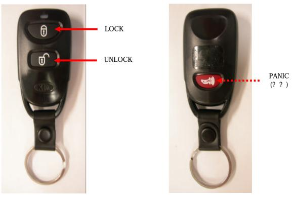
You can lock and unlock your vehicle with the remote transmitter.
