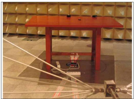
• Front View of Radiated Emission (Biconical Antenna)
