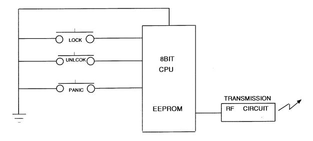
figure 3.1 block diagram of the transmitter
