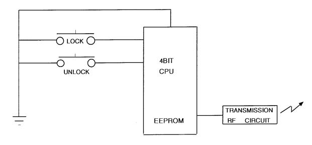
figure 3.1 block diagram of the transmitter
