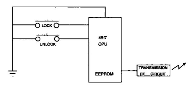
figure 3.1 block diagram of the transmitter
