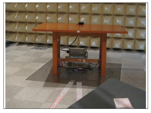
• Front View of Radiated Emission (Logperiodic Antenna)
