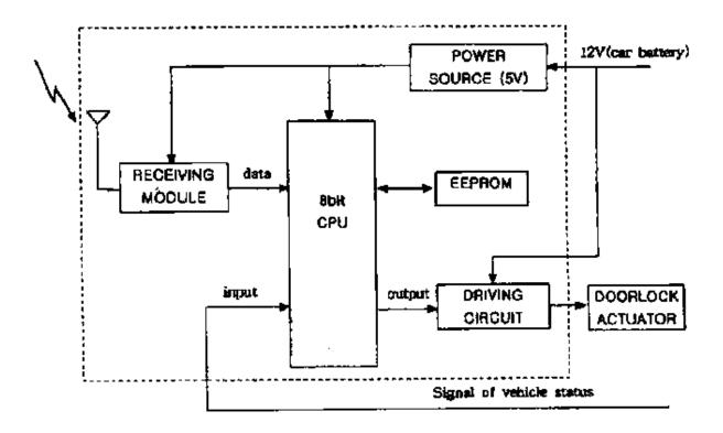
figure 3.1 block diagram of the receiver
