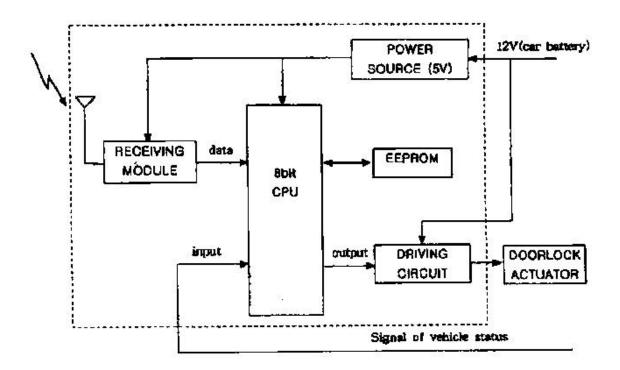
figure 3.1 block diagram of the receiver
