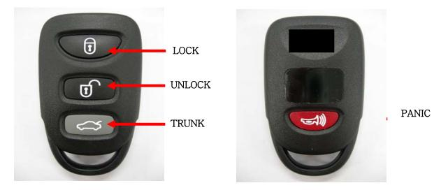
You can lock and unlock your vehicle with the remote transmitter.
