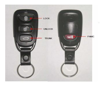
You can lock and unlock your vehicle with the remote transmitter.
