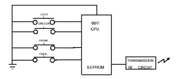
figure 3.1 block diagram of the transmitter
