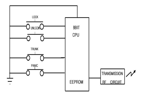
figure 3.1 block diagram of the transmitter
