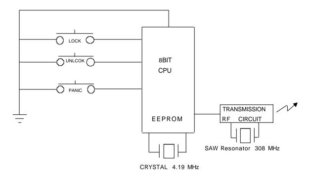
figure 3.1 block diagram of the transmitter
