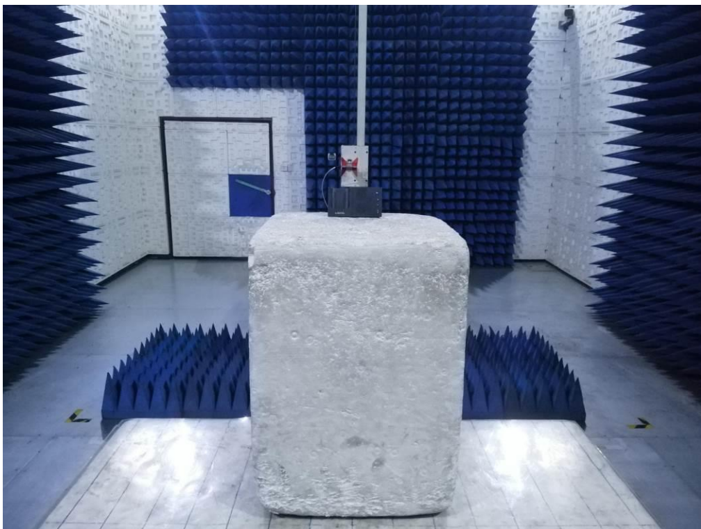
RADIATED EMISSION TEST SETUP ABOVE 1GHz
