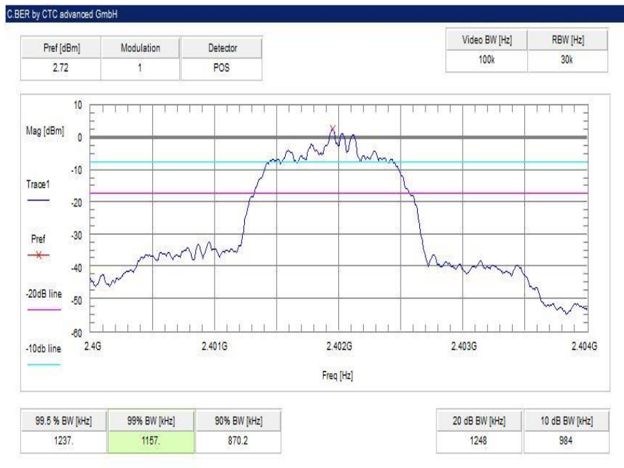
Plot 4: lowest channel – 2402 MHz, Pi / DQPSK modulation
