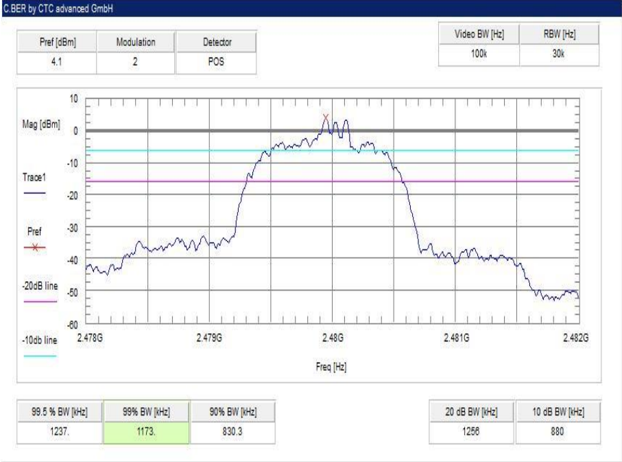
Plot 9: highest channel – 2480 MHz, 8 DPSK modulation
