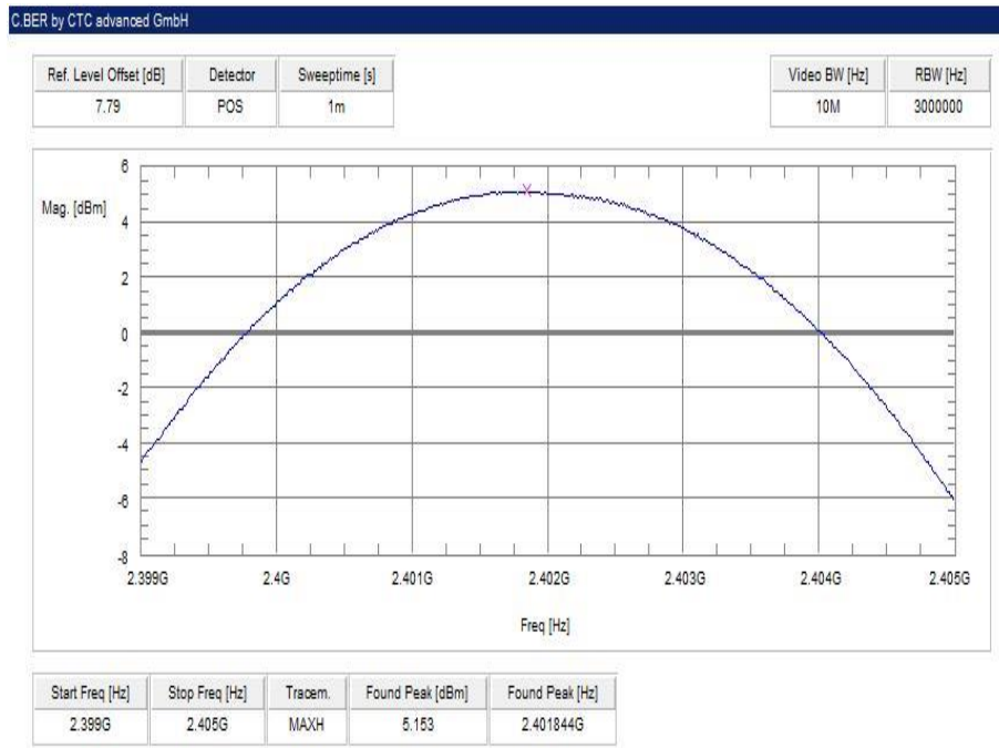
Plot 4: lowest channel – 2402 MHz, Pi / DQPSK modulation
