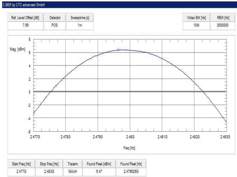
Plot 6: highest channel – 2480 MHz, Pi / DQPSK modulation
