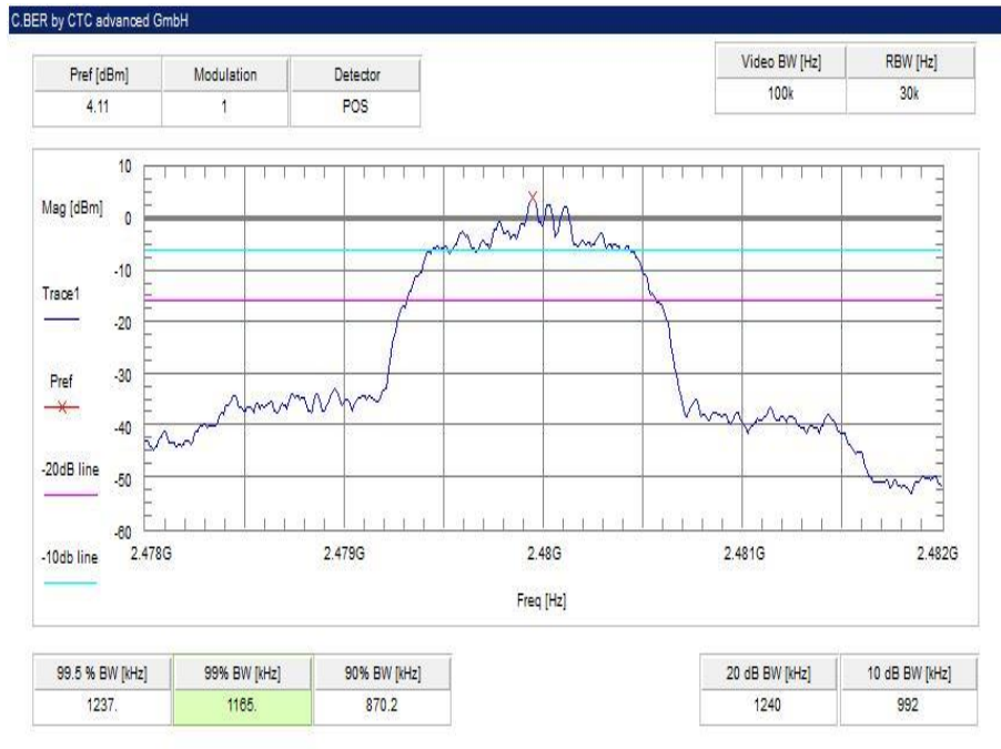
Plot 6: highest channel – 2480 MHz, Pi / DQPSK modulation
