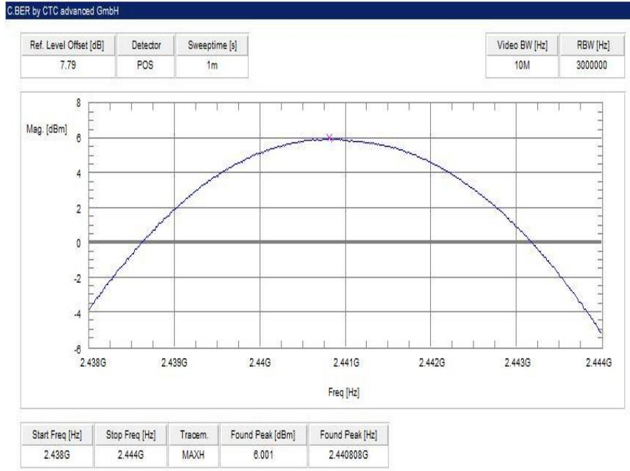
Plot 5: middle channel – 2441 MHz, Pi / DQPSK modulation
