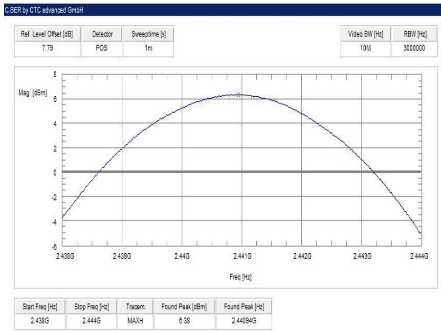
Plot 8: middle channel – 2441 MHz, 8 DPSK modulation
