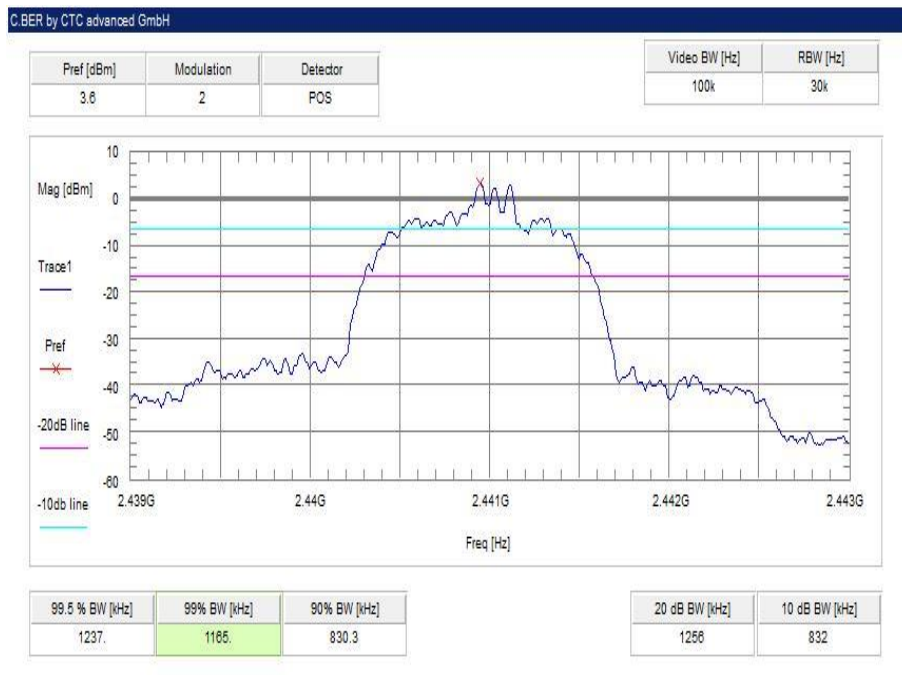
Plot 8: middle channel – 2441 MHz, 8 DPSK modulation
