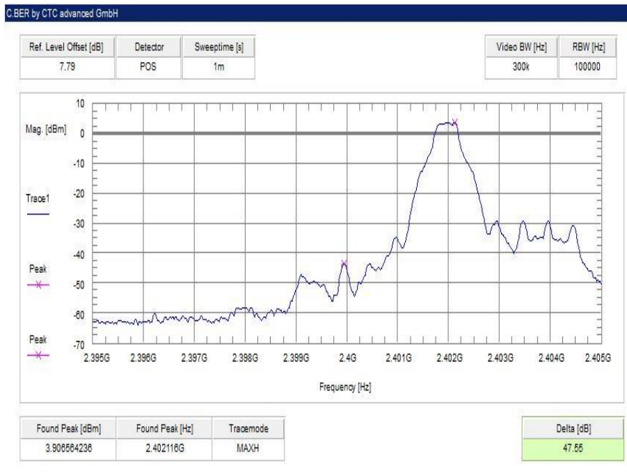
Plot 3: Lower band edge – hopping off, GFSK modulation
