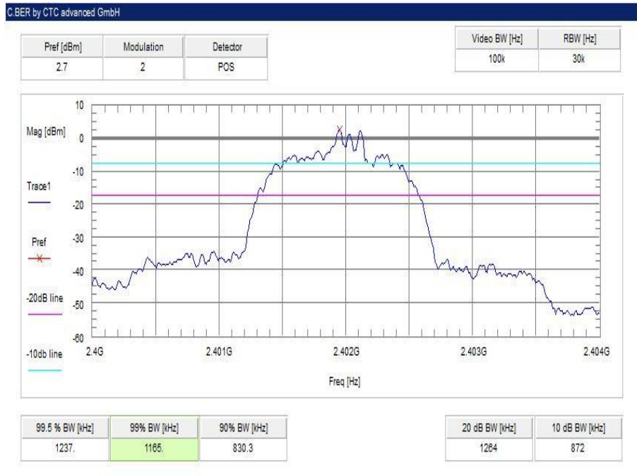
Plot 7: lowest channel – 2402 MHz, 8 DPSK modulation
