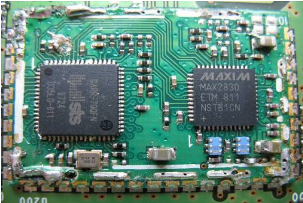
Photo 15: (sample for radiated measurements) Module under the shield plate
