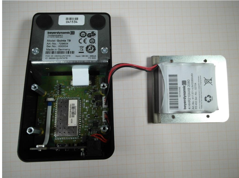
Photo 1 (EUT - battery pack & main board):
