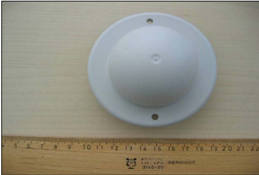
Photo 31: Omnidirectional antenna (CA Q14)
