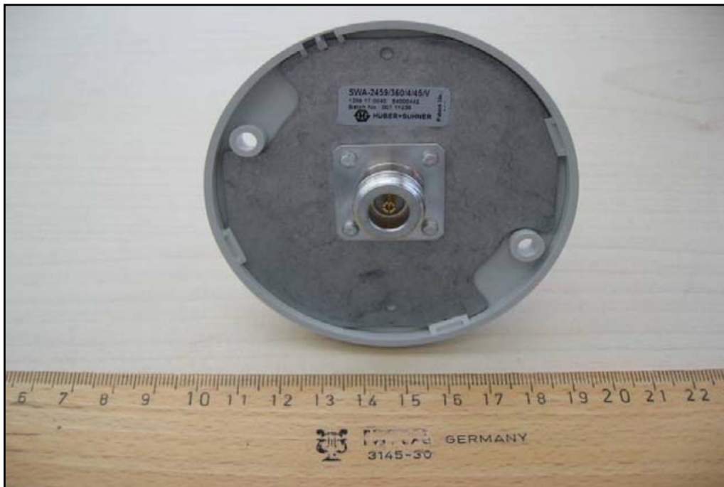
Photo 32: Omnidirectional antenna (CA Q14)
