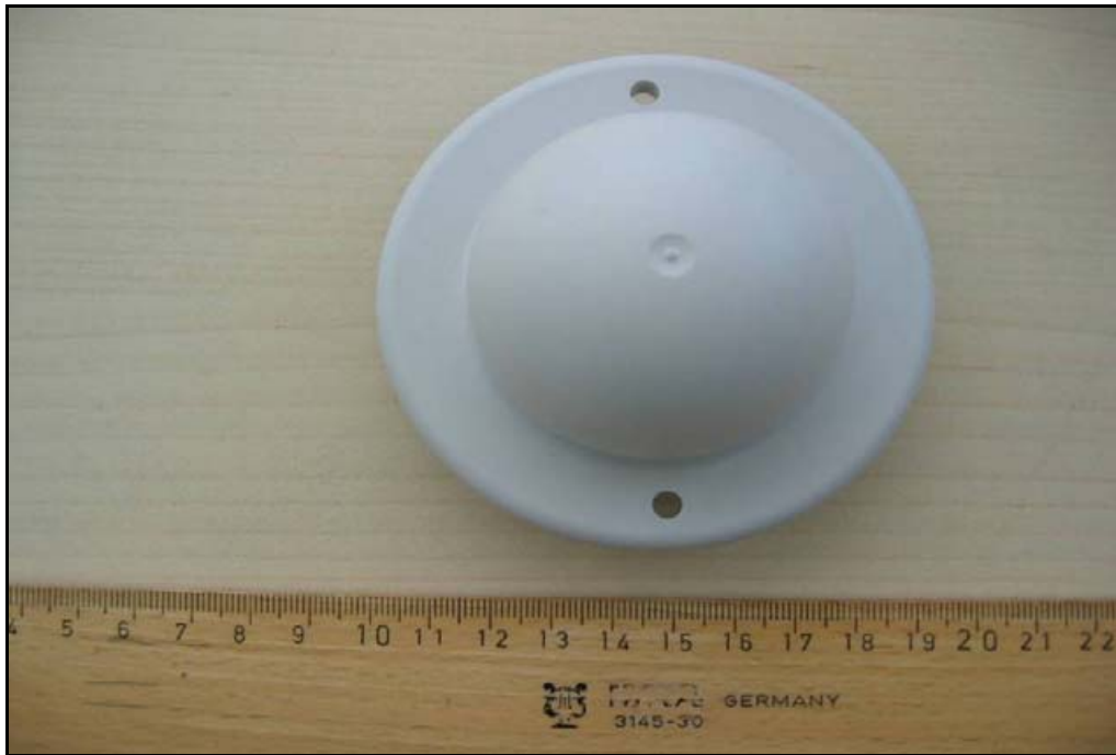
Photo 31: Omnidirectional antenna (CA Q14)
