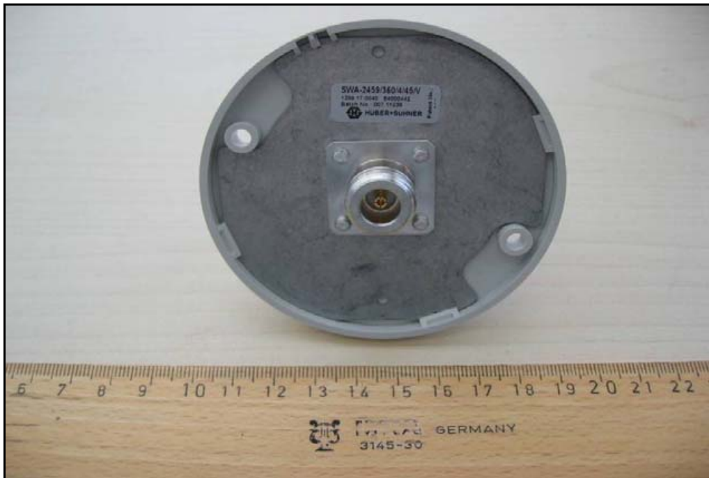
Photo 32: Omnidirectional antenna (CA Q14)
